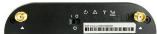
ON-OFF / LEDs / SIGNAL STRENGTH IBR650
