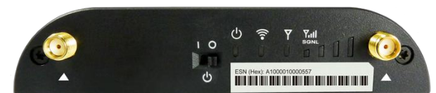
ON-OFF / LEDs / SIGNAL STRENGTH IBR600
